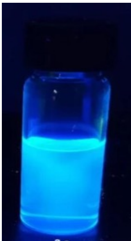
Figure: Blue emission N-CQDs under UV light
